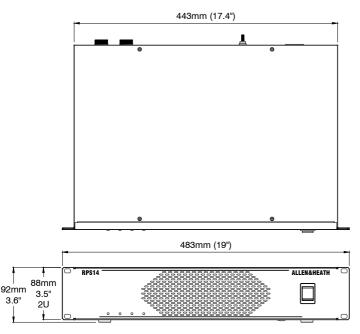
The **RPS14** is supplied ready for use free standing. For rack mounting remove and retain the four rubber feet.
